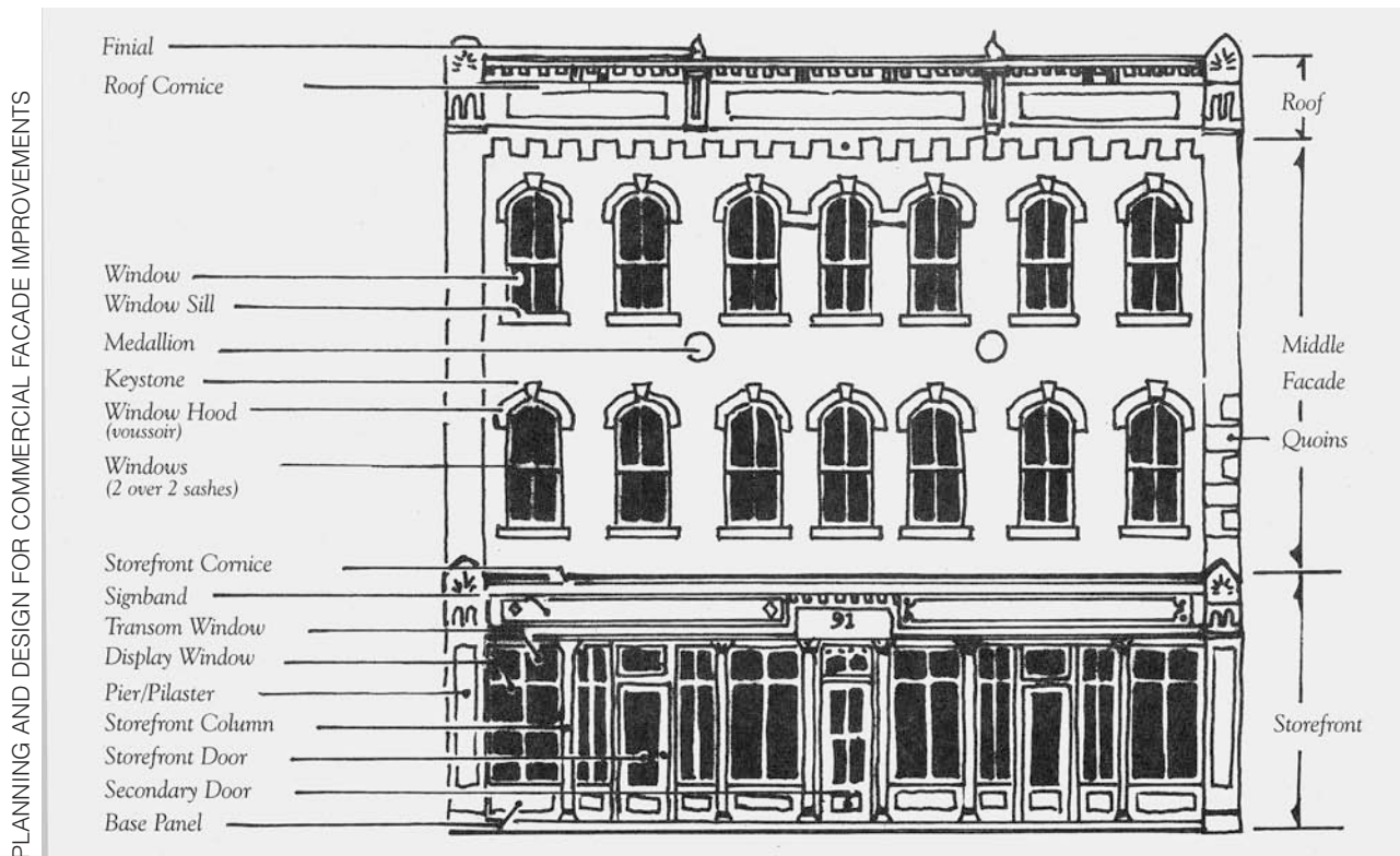
Components of a Commercial Building
